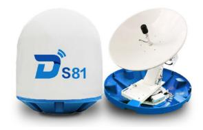
Ditel S81 is a marine satellite TV antenna system that has excellent satellite signal reception capability with a 83cm (32.70") reflector. It is widely used in anywhere in the world as long as the area of Minimum EIRP is over 44dBW. 3-axis is preferred in the vicinity of the equator.
